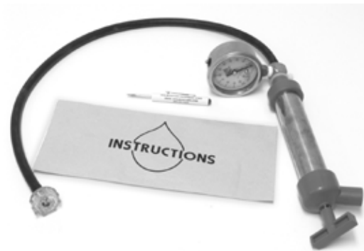
2005G2, Vacuum Test Hand Pump (shown with tubing and service cap for servicing tensiometers)
