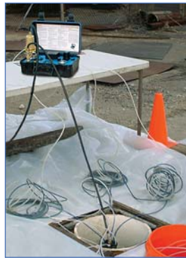
An EPA regulated site in Northeast, USA. This multilevel array allowed a sampling team to purge and sample from 40 monitoring zones across 10 borehole locations in just 4 days. These Waterloo Systems were installed in overburden using preinstalled casing.
