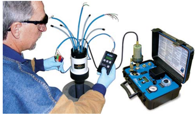
Taking pressure measurements with Model 404 Geokon Vibrating Wire Readout
