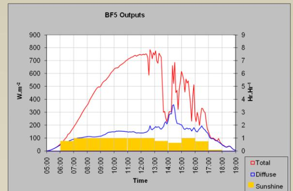
Illustration of BF5 output showing Total and Diffuse radiation and Sunshine status (hours/hour)
