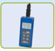
Technical data HD2 Convenient one-hand operation. The multi-line LCD display shows all information at a glance 4,8V-DC, 2000mAh battery Power supply: capacity. Full battery for up to 1,500 measuring cycles sufficient Resolution: 0,01% Calibration (on sensor) Weatherproof, robust aluminium diecast (IP67) 150 x 64 x 36mm (Length x Dimensions: width x height), Weight: 437g
