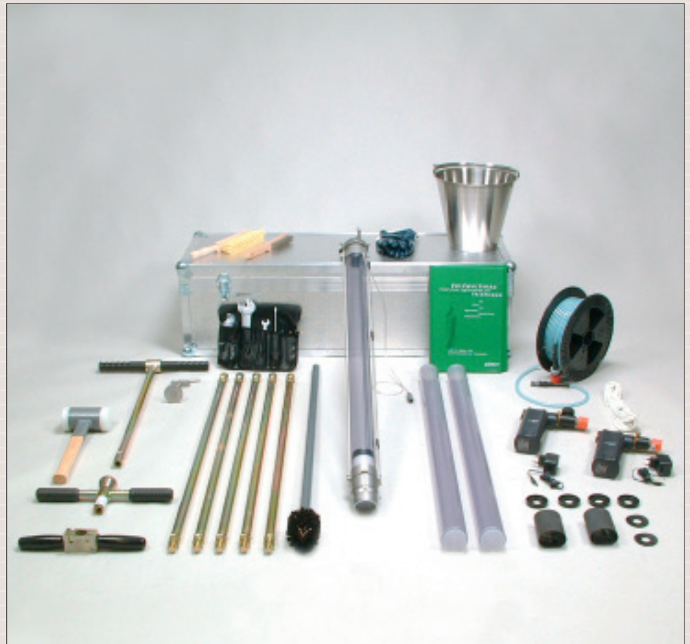
Sediment core sampler type Beeker, complete basic set (04.23.SA)
