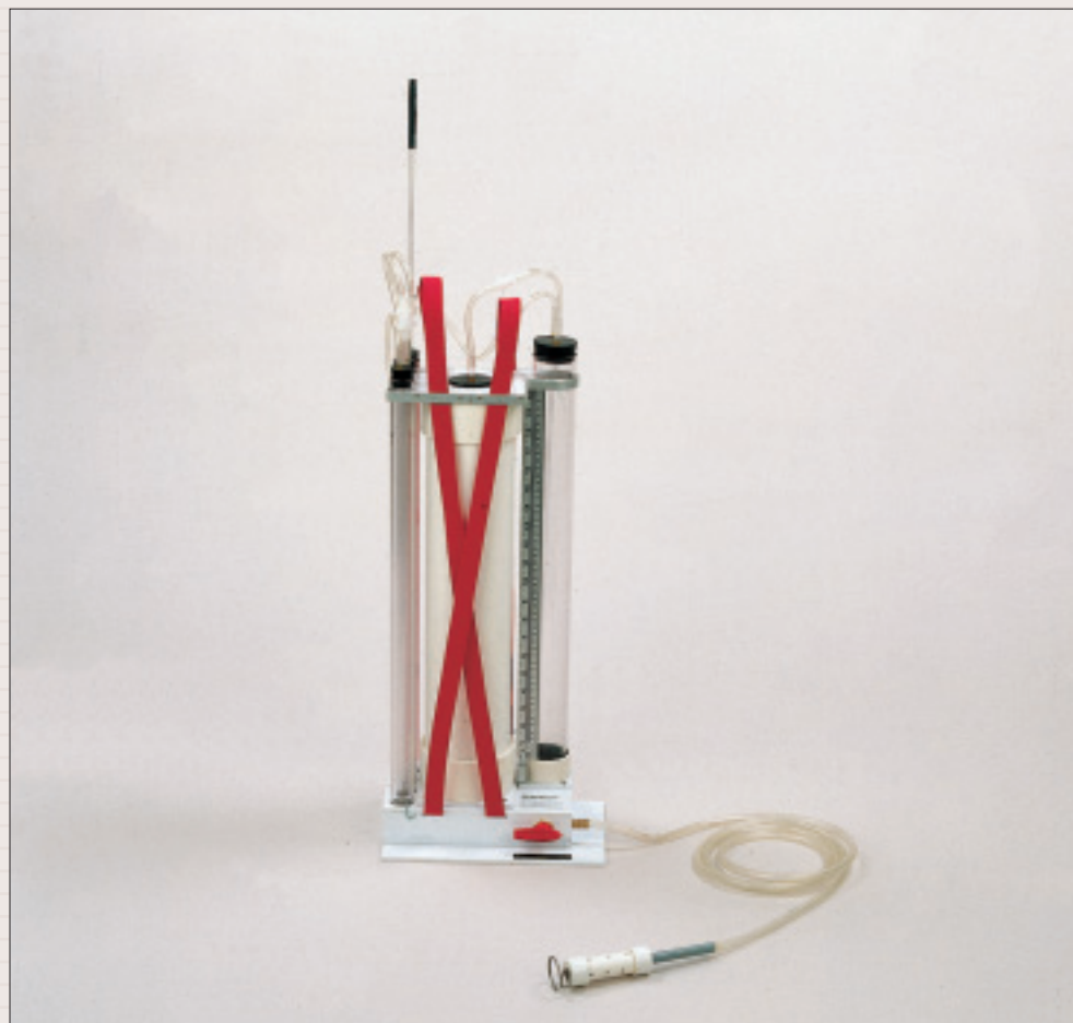
Ksat constant head permeameter
