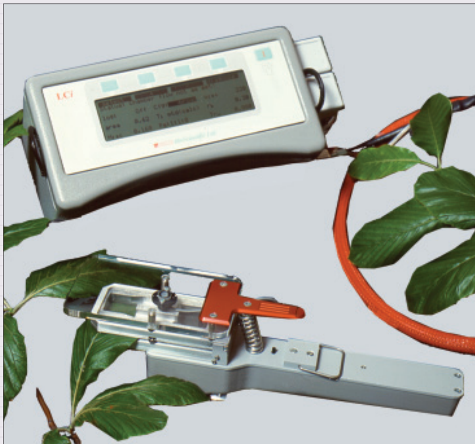
Portable system for CO 2 and transpiration measurements
