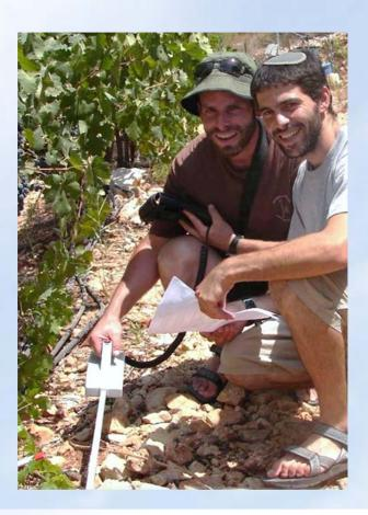
It was important to determine that LAI measurements were reliable and accurate and so in order to verify the accuracy of SunScan LAI measurements, leaves were removed from a total of eighteen 2m sections of grapevine and measured with an area meter.
