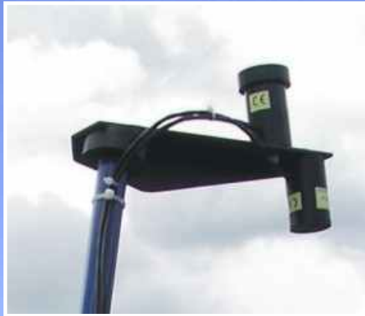
Sensors mounted for measuring incident & reflected light
