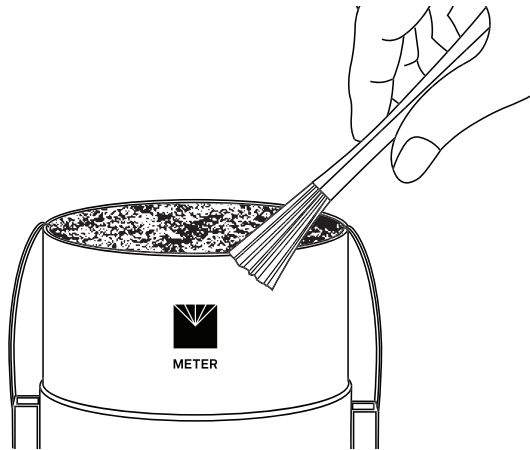
Figure 49 Fix and clean the soil sampling ring
