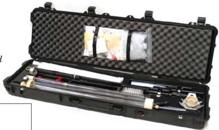
Fig. 1b - Guelph Permeameter Carrying case
