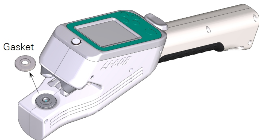
Figure 8-2. Removing the gasket.
