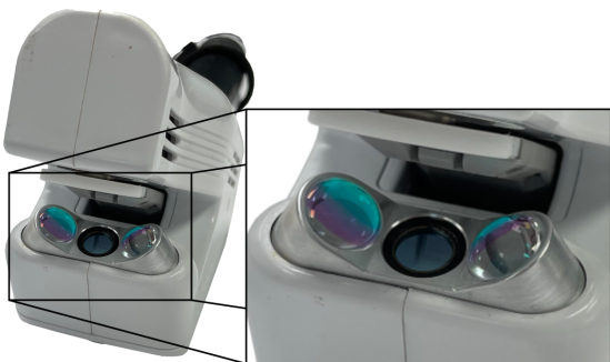
Figure 8-4. The fluorometer LEDs and fluorescence detector.
