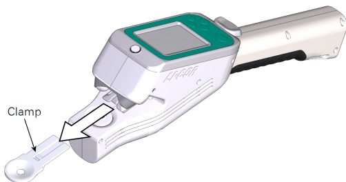
Figure 8-1. Removing the clamp.
