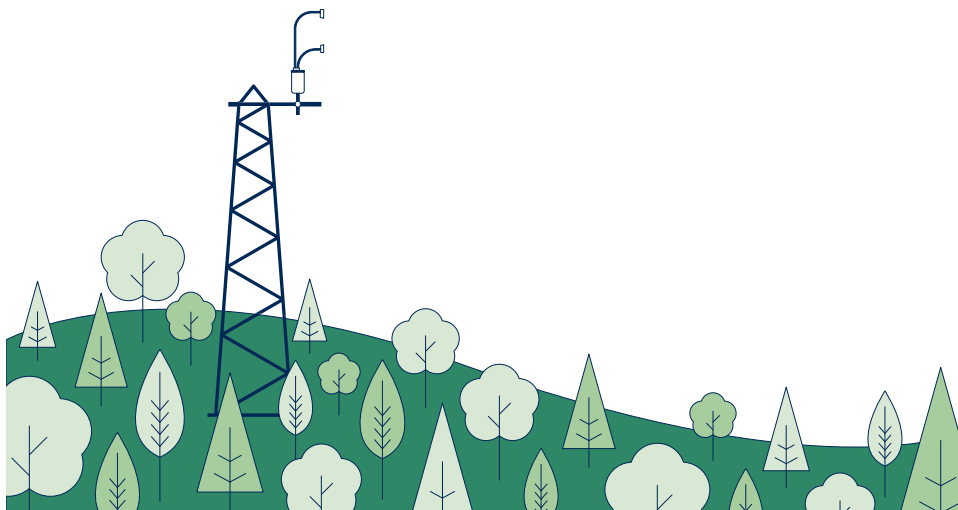
Figure 3-7. The LI-710 should be at least 3 meters above the top of orchards, woodland, and forest canopies.
