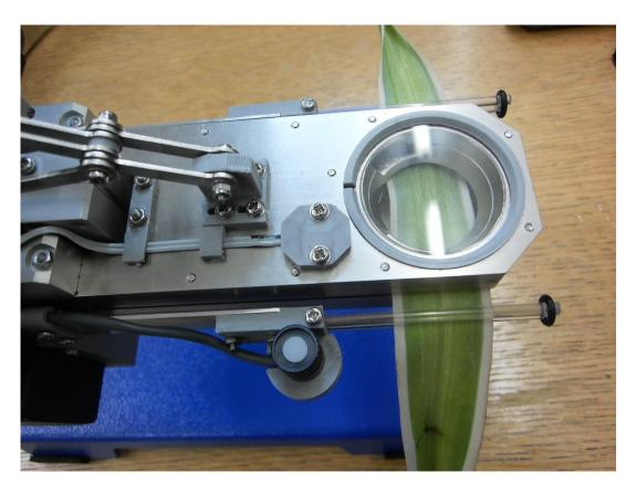
The transparent leaf guides are designed to hold the leaf so that it maintains a constant position relative to the closed position of the jaws, even when they are open.
