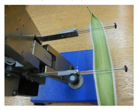
They are retained by M2 pan head screws (shown, arrowed), which should by tightened till they just grip the guides. The guides may be replaced if they become damaged, and may be cut shorter using sharp side
