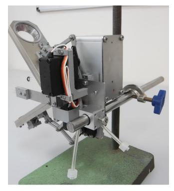
The chamber may also be attached to horizontal rods from the back or side. To do this it is necessary to remove, rotate and refit the mounting block
