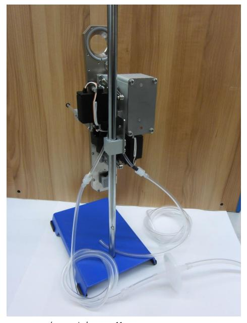
If the chamber is warm and the surrounding air is cool it is possible that the outlet pipe might have droplets of water condensing in it. Connect the outlet pipe to the controller inlet via the supplied hydrophobic filter 630-976 to catch these droplets that would otherwise cause damage to the gas analysis system. Fit the filter at the controller end of the white sleeved pipe which supplies air to the analyser.
