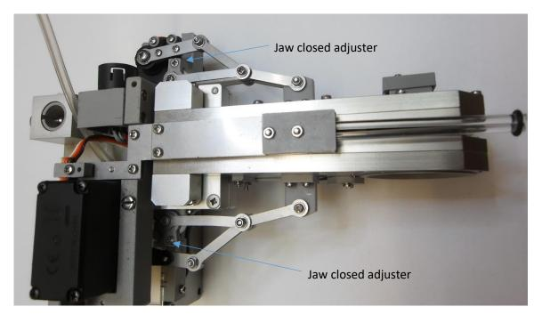
When the chamber is connected to a controller, and has been closed by software request, these adjusters can be moved to make small changes to ensure that the gaskets are touching with no air gaps. Make this adjustment before using it on a leaf.
