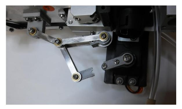
The plastic servo arms APS138 are intended to break as in the photo above if excessive forces are placed on the jaws, to prevent damage to the servo mechanism and to protect the user. The APS138 arms break at a closed clamp force of approximately 1.5 kg at the leaf position. They are supplied in the spares kit, are available as spares from ADC and are easily replaced using a pozidrive #1 screwdriver, a 5.5mm and a 4mm spanner or pliers.
