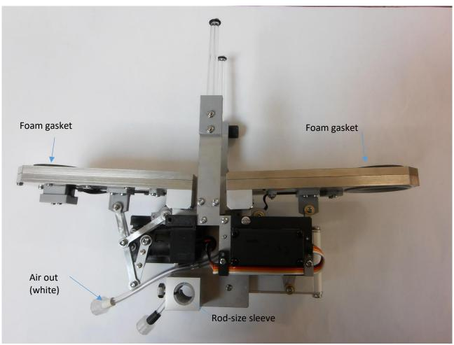
The chamber is 27cm between jaw tips when open.
