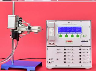
The **APS chamber** has two hinged jaws that automatically close onto a leaf to measure the photosynthetic rate.
