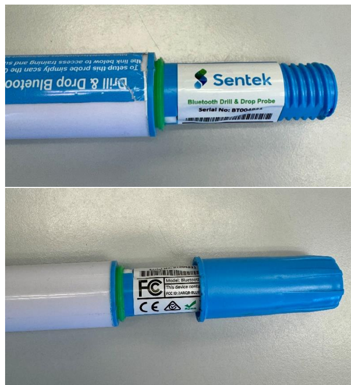
Bluetooth Probe head incorporating battery compartment, antenna, and serial number
