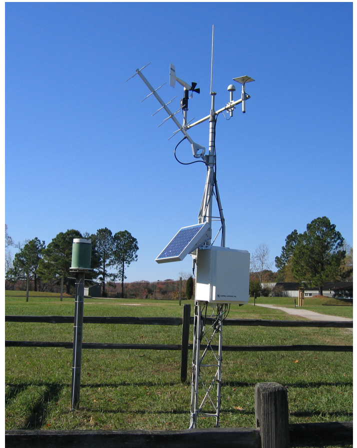
This station for the National Estuarine Research Reserve (NERR) in Virginia transmits data via our GOES satellite transmitter.
