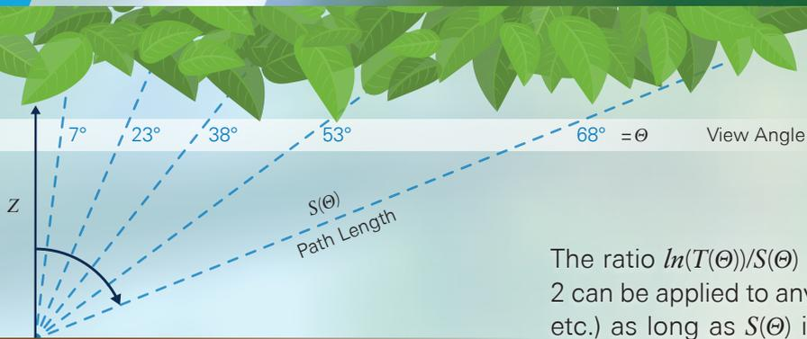
The path length of the optical sensor's view through a full cover canopy varies by view angle.
