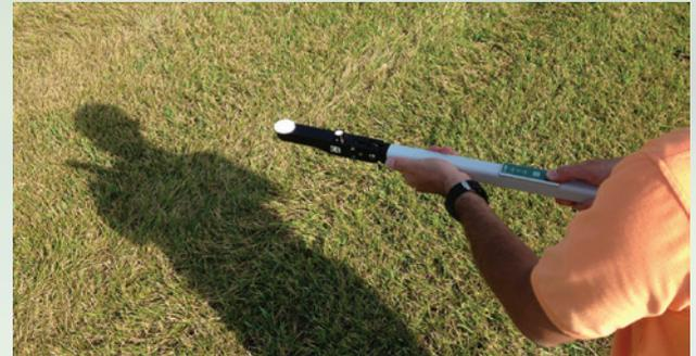
Using an optical sensor with diffuser cap to measure sky radiation properties for light scattering correction.
