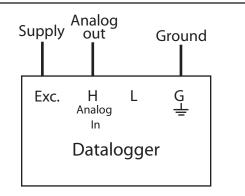
If your MPS-1 is equipped with the standard 3.5mm plug, and you wish to connect it to a non-Decagon datalogger, you have two options. First, you can clip off the plug on the sensor cable, strip and tin the wires, and wire it directly into the datalogger. This has the advantage of creating a direct connection with no chance of the sensor becoming un-plugged; however, it then cannot be used in the future with a Decagon Em50 or Em50R logger.
