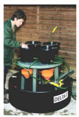
Australia, the Root Washer consists of four buckets each with a central overflow pipe and two water jets in the base. The water swirls around and up, teasing roots and soil apart. Fine roots in the outflow are collected in a 500 micron mesh filter; those remaining in the bucket are poured through the filter. Depending on the soil type and sample volume, about 10 samples per hour can be washed.
