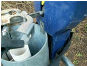
Fig. 2 Actuator hooked on the upper rim
