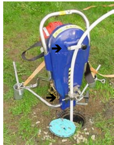
Fig. 12 Tubing fixed in upper and lower tube guide
