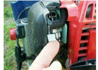
Fig. 15 Putting choke in position " Choke "
