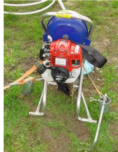
Fig. 7 Two anchors are used to install the actuator
