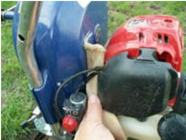
Fig. 5 Pass strap behind electric cables
