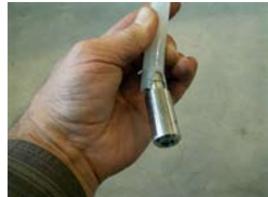
Fig. 11 Removing a valve
