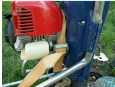
Fig. 6 Pull strap between engine and crankcase
