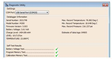
You may be able to diagnose what has caused your battery to drain more quickly than expected, by using the Levelogger Software Diagnostic Utility. The Utility will display the temperatures your Levelogger has been exposed to, an estimate of the number of logs that were taken, as well as the battery voltage and charge levels.
