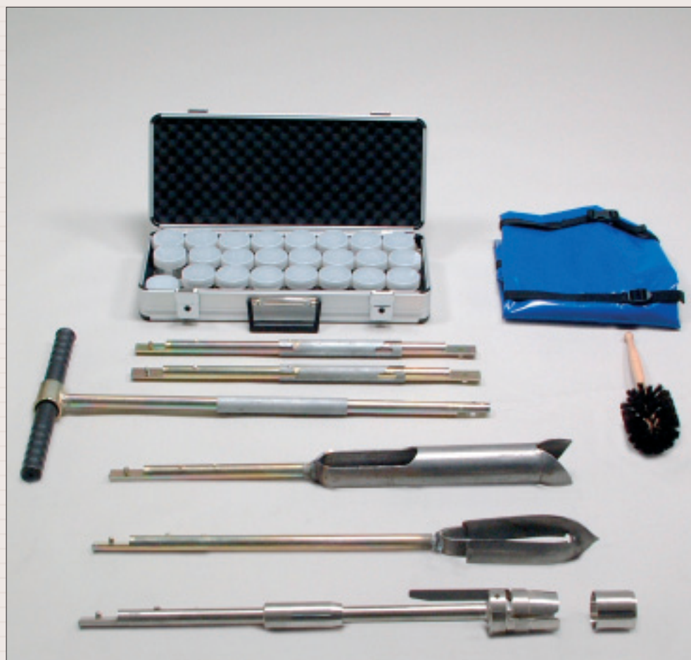
Sample ring kit for soft soils
