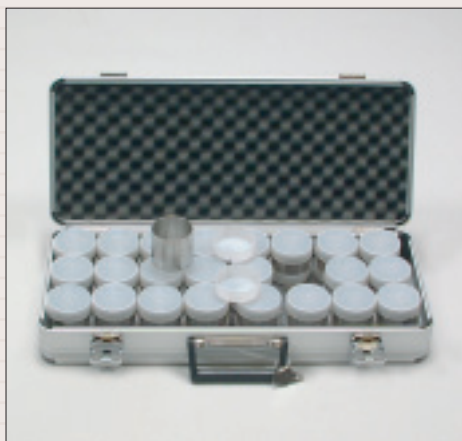
Soil sample rings in case
