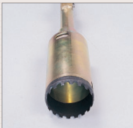
Drilling-crown, extruder in upper position
