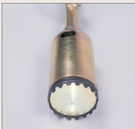
Drilling-crown, extruder in lower position
