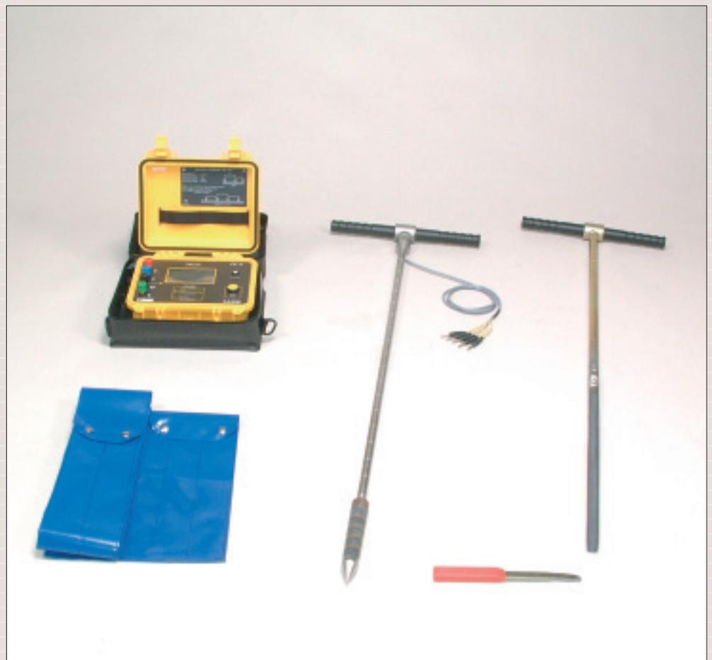
EC-probe for soil salinity measurements, standard set
