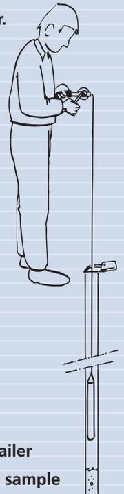
A stainless steel bailer sampler is used to sample open water.
