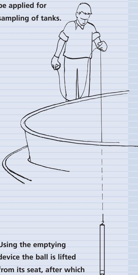
Using the emptying device the ball is lifted from its seat, after which the sampler is drained.
