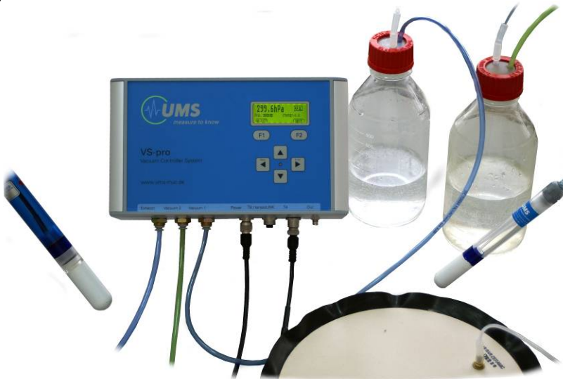
Abb. 2.1: Parts of a soil water sampling system
