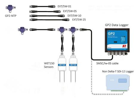
Cables can be joined via extension cables and T-connectors. Maximum cable lengths depend on configuration details. As an example, 200m with 10 WET150s each connected via a 5m extension cable works reliably with the GP2 Data Logger.
